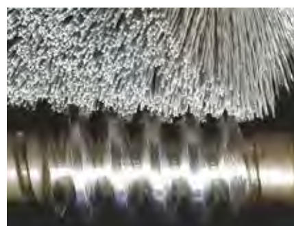
Pulire profili dentati / Crown profiles cleaning
