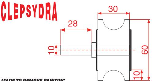
MADE TO REMOVE PAINTING FROM RAILINGS, TO CLEAN PIPES AND REINFORCING
